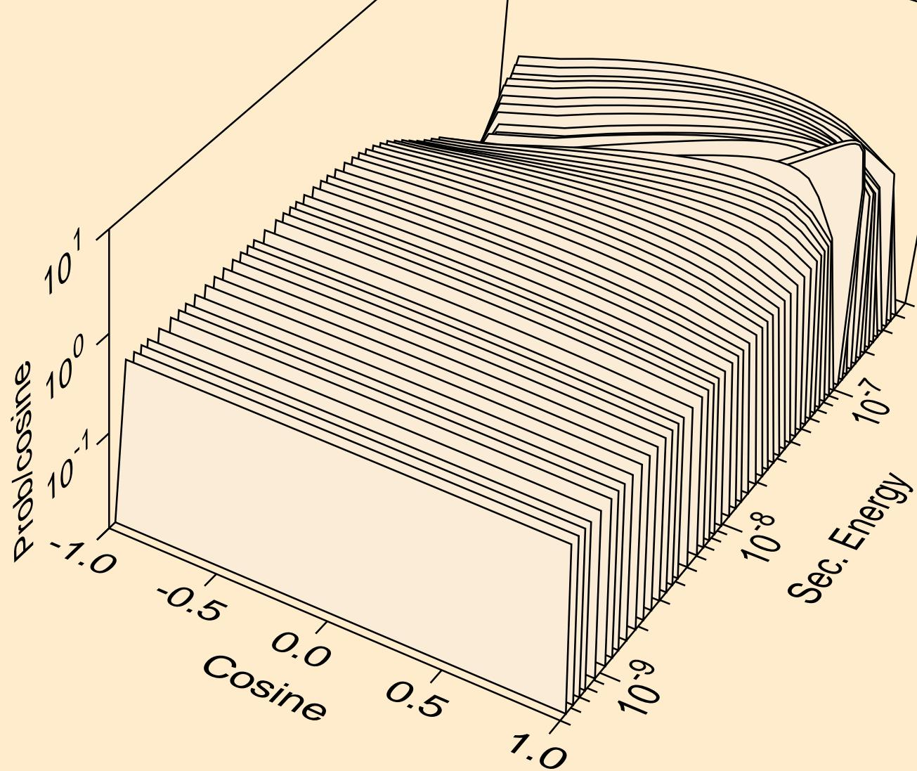
1-H-1 IN H<sub>2</sub>O AT 293.6K FROM ENDF/B-VII USING CONTINUOUS
