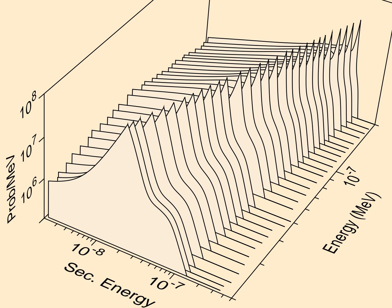
1-H-1 IN H<sub>2</sub>O AT 293.6K FROM ENDF/B-VII USING CONTINUOUS
