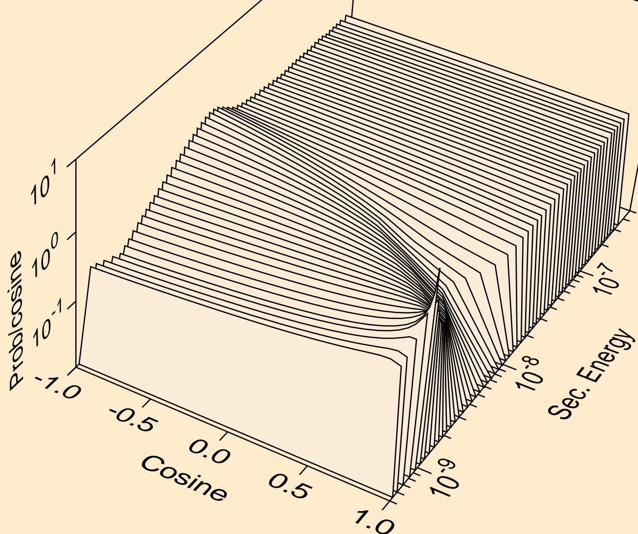
1-H-1 IN H<sub>2</sub>O AT 293.6K FROM ENDF/B-VII USING CONTINUOUS
