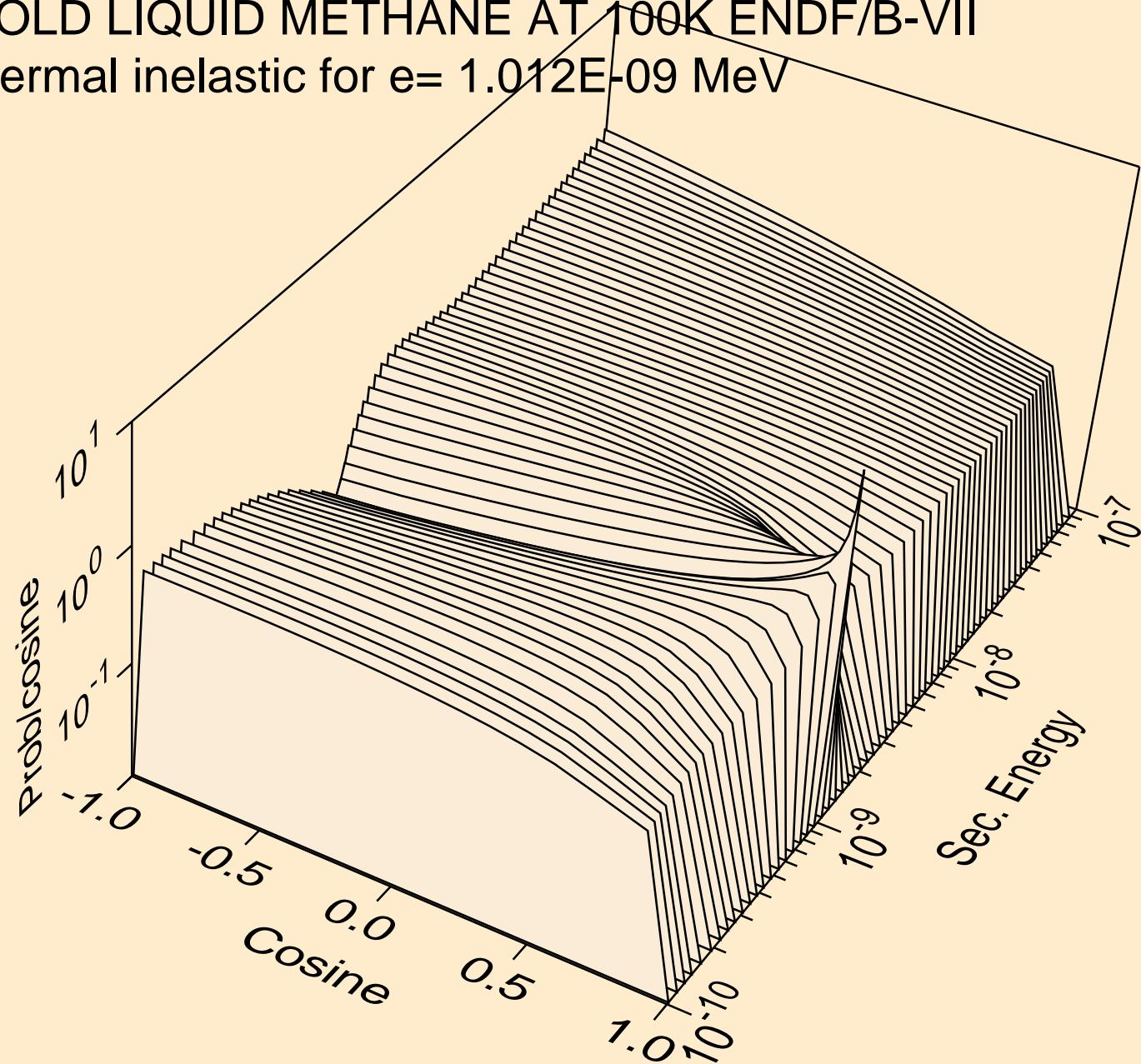
COLD LIQUID METHANE AT 100K ENDF/B-VII
