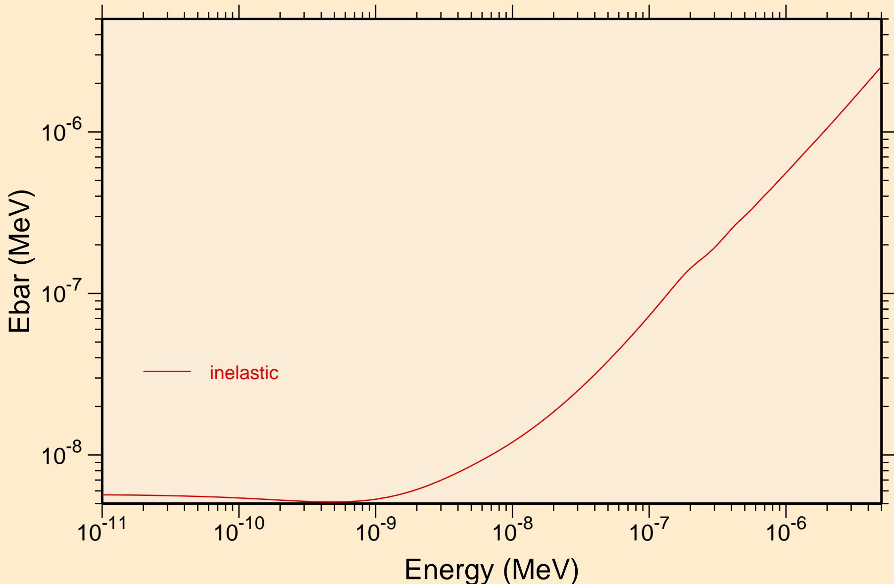
COLD LIQUID METHANE AT 100K ENDF/B-VII
