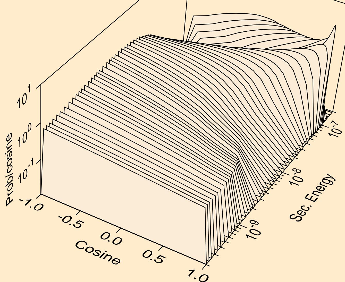
COLD LIQUID METHANE AT 100K ENDF/B-VII
