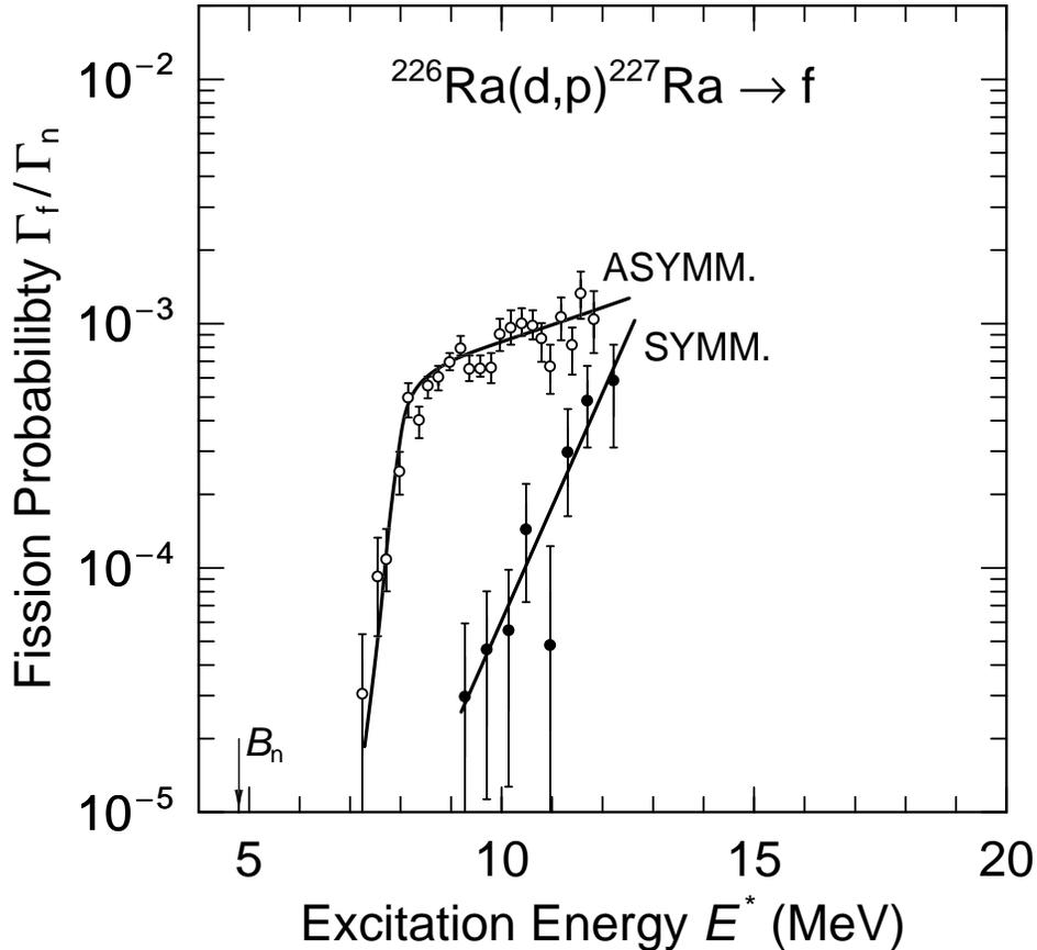
Figure 1: Fission probability data show different thresholds for mass-asymmetric and mass-symmetric fission near  $^{227}\text{Ra}$ . The figure is based on a figure in Ref. [1].
