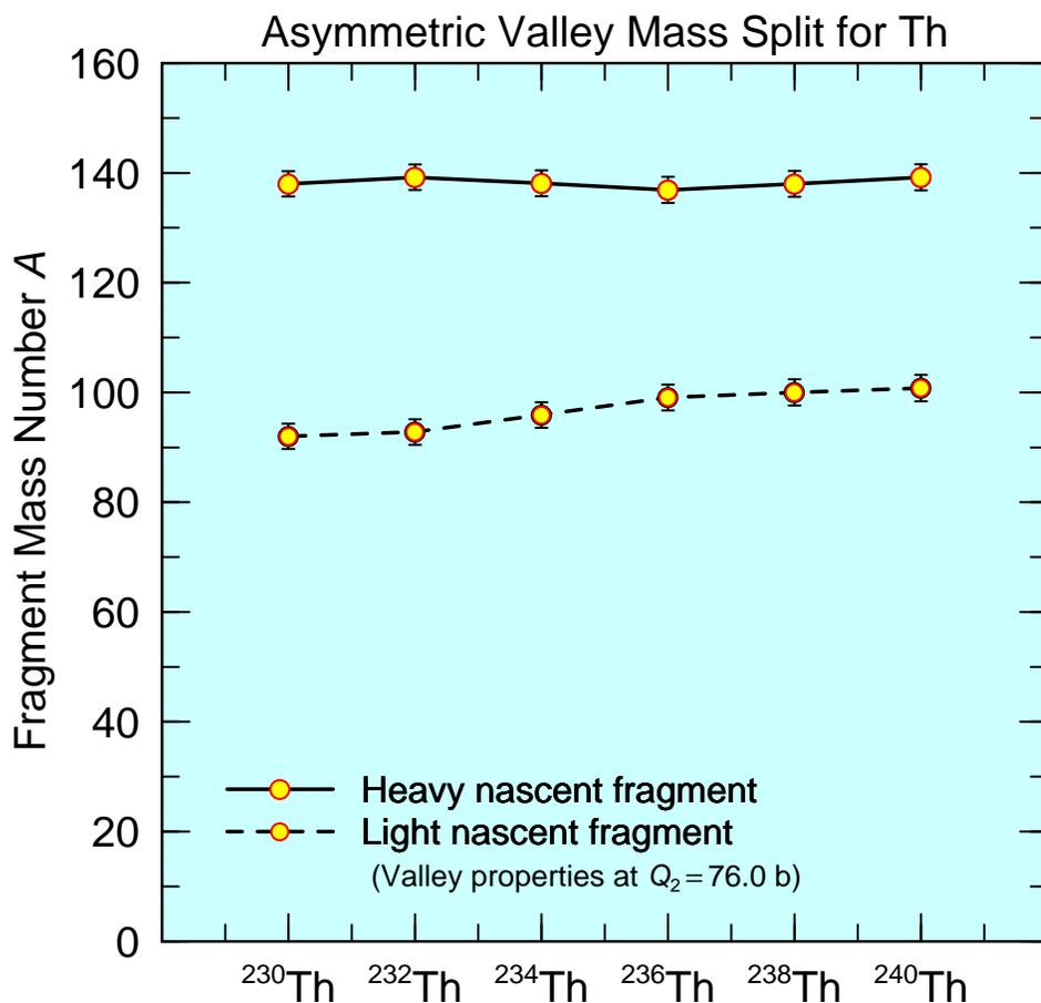
Figure 10: Mass divisions in asymmetric fission for a sequence of Th isotopes from  $^{230}\text{Th}$  to  $^{240}\text{Th}$ . The results are in excellent agreement with the experimental observation of a constant-mass heavy fragment at mass number  $A \approx 140$  and a light fragment mass corresponding to the remainder of the mass of the original fissioning nucleus.
