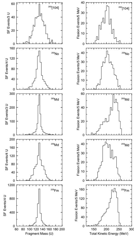
Figure 3: Experimental fission-fragment mass and kinetic-energy distributions for the fission of nuclei close to  $^{264}\text{Fm}$ , whose symmetric fragments are doubly magic. The structures of these distributions reflect the valleys, ridges, minima, and saddle points of the underlying nuclear potential-energy surfaces. Taken from Ref. [4].
