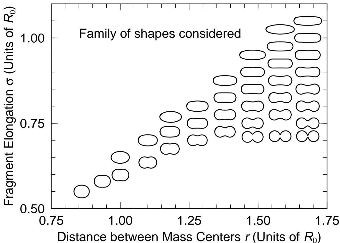
Figure 4: Typical nuclear shapes for which fission potential-energy surfaces are calculated. The selected shapes allow fission into both compact spherical fragments with high kinetic energies and elongated fragments with normal kinetic energies.
