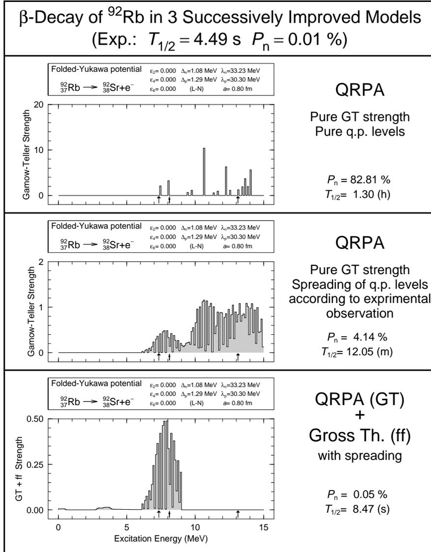
Figure 2: Calculated  $\beta$ -strength functions, corresponding half-lives and delayed-neutron emission probabilities for  $^{92}\text{Rb}$  in three successively enhanced models. The narrow arrow indicates the  $Q_\beta$  value, the wide arrows successive neutron-separation energies; the lowest arrow  $S_{1n}$ , the second lowest  $S_{2n}$ , and so on. The results are further discussed in the text.
