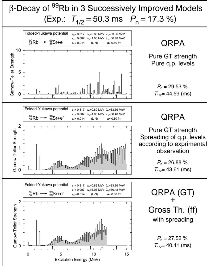
Figure 1: Calculated  $\beta$ -strength functions, corresponding half-lives and delayed-neutron emission probabilities for  $^{99}\text{Rb}$  in three successively enhanced models. The narrow arrow indicates the  $Q_\beta$  value, the wide arrows successive neutron-separation energies; the lowest arrow  $S_{1n}$ , the second lowest  $S_{2n}$ , and so on. The results are further discussed in the text.
