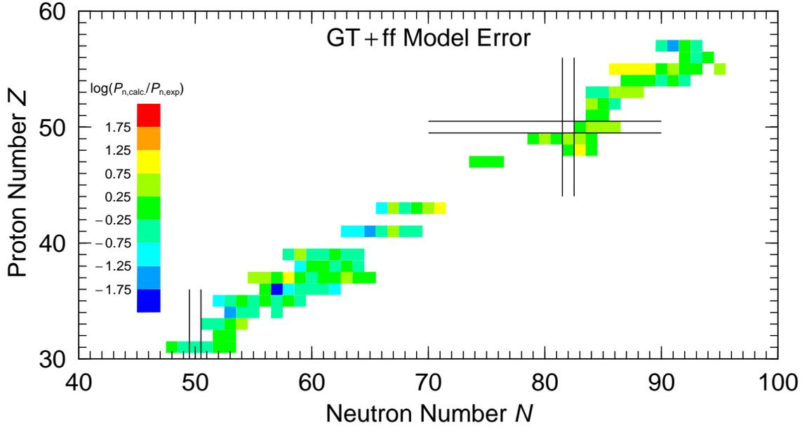
Figure 9: “Nuclear-chart” plot of the ratio of calculated to experimental  $\beta^-$ -delayed neutron-emission probabilities for nuclei in the fission-fragment region. In this case first-forbidden transitions, as given by the statistical gross theory, are taken into account.
