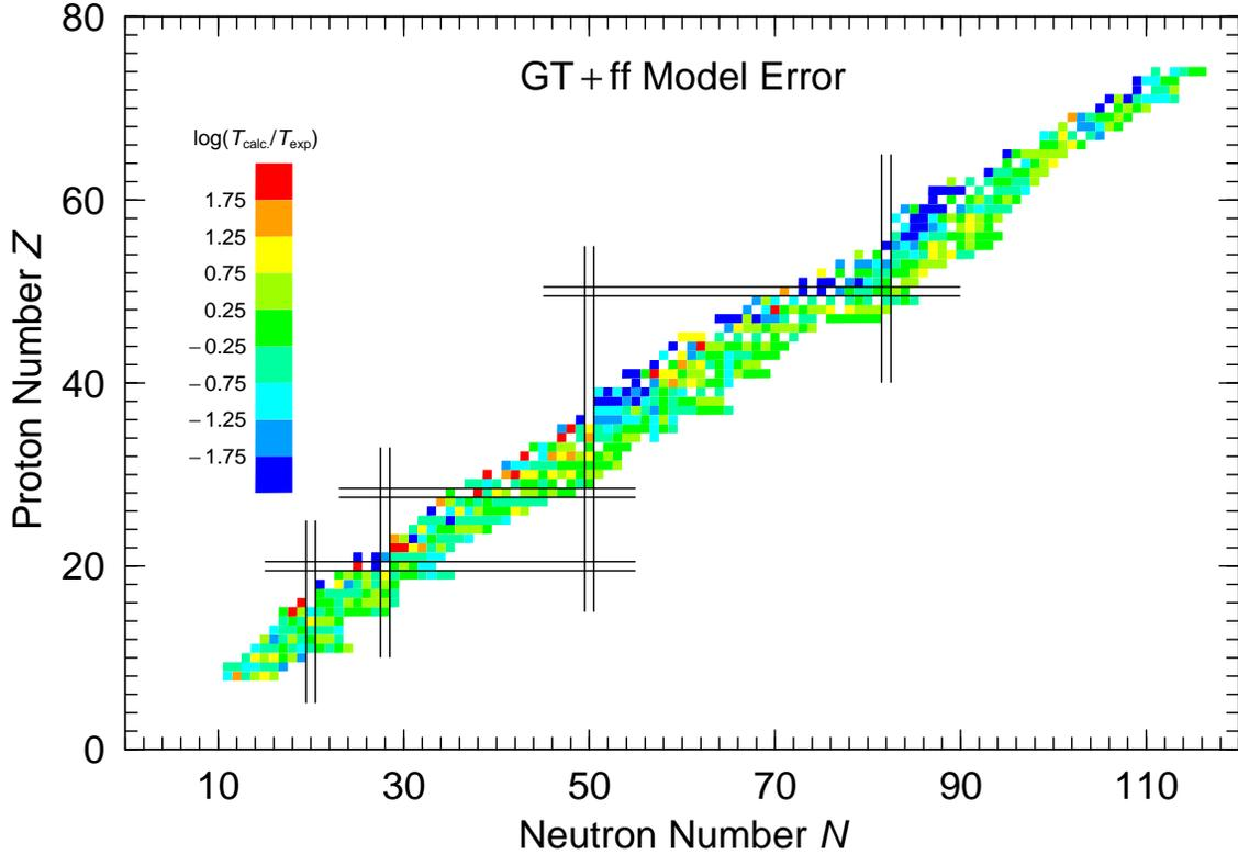
Figure 7: “Nuclear-chart” plot of the ratio of calculated to experimental  $\beta^-$ -decay half-lives for nuclei from  $^{16}\text{O}$  to the heaviest known. In this case first-forbidden transitions, as given by the statistical gross theory, are taken into account.
