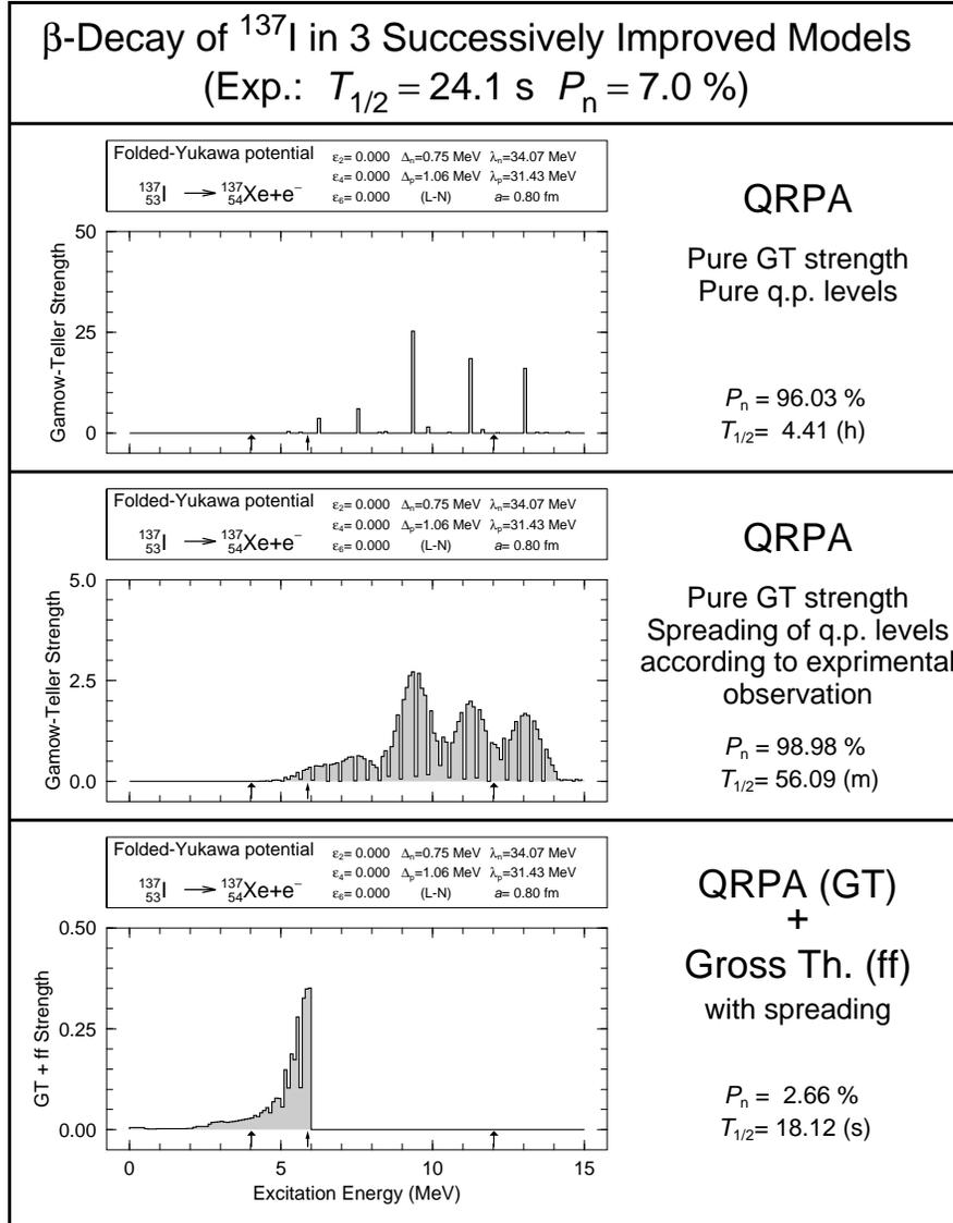
Figure 3: Calculated  $\beta$ -strength functions, corresponding half-lives and delayed-neutron emission probabilities for  $^{137}\text{I}$  in three successively enhanced models. The narrow arrow indicates the  $Q_\beta$  value, the wide arrows successive neutron-separation energies; the lowest arrow  $S_{1n}$ , the second lowest  $S_{2n}$ , and so on. The results are further discussed in the text.
