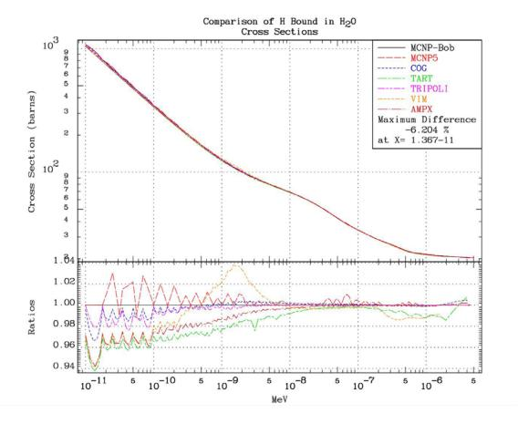
The scallops seen in the above plot are the result of each code using a different energy grid for its cross section. For a convex cross section generally using fewer energy points will cause scallops pointing upward, as in the case of the MCNP5 ratios at low energies in the above plot; using more energy points will cause scallops pointing downward, as in the case of the AMPX, TART and VIM ratios at low energy.
