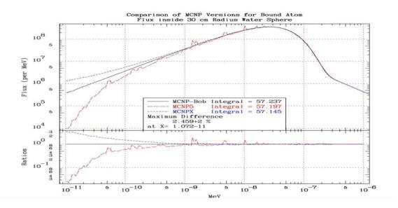
Sometimes it is difficult to judge the actual magnitude of differences on log scaled plots, so below we show a comparison of the spectra calculated by the three codes across the entire peak of the thermal spectrum. Here we can more clearly see the smoothing effect of MCNPX, and the spike of MCNP5. The second figure shows that MCNPX still differs from MCNP-Bob by a significant amount; not the factors of 2 seen for MCNP5, but still by up to 10%.
