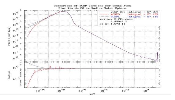
The second plot shows perfect agreement above 10 eV (10<sup>-5</sup> MeV on the plot). Based on the perfect agreement that we saw earlier using free atom data, this is not surprising, since the bound data only extend up to 4 eV, and we expect the results using free and bound data to be identical above this energy.
