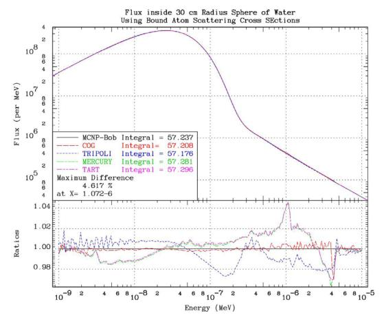
Overall the agreement is very good. If we look only at the upper part of these figures it is hard to see any differences at all (to within the thickness of the lines). Only the lower part of these figures showing the ratios allows us to find the per-cent differences. Again, remember that the small differences seen here were achieved only after several iterations to improve the agreement between code results.
