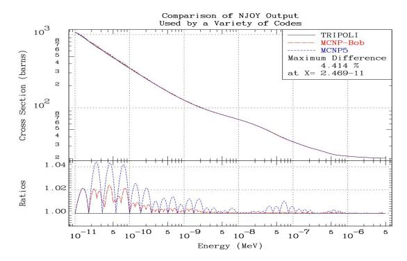
This is an excellent example of a processing code "dial" that can affect results, as mentioned in the introduction; here it appears that the TRIPOLI cross sections are based on the user telling the NJOY nuclear data processing code to produce many more energy points.
