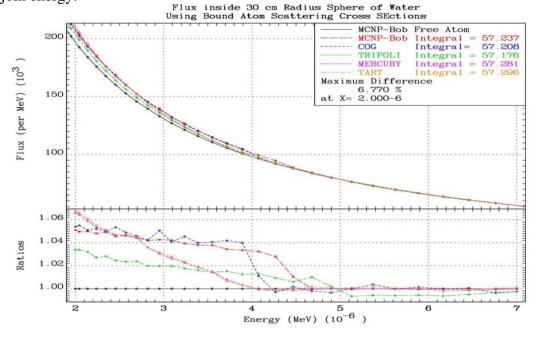
As mentioned above, log scaling can often mask the real magnitude of differences, so below we show the important energy range around the peak of the thermal spectrum. Note that near the peak of the spectrum all of the codes agree well at the 1% level. This agreement is not great, and certainly no where near as good using free atom, but it is much better than what one might expect by looking at a wider energy range.
