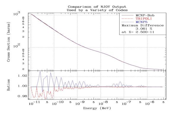
As mentioned earlier, the scallops on these plots are due to the use of different energy grids. Based on the above plot it appears that we are using the wrong code as the standard to ratio everything else to, as we will see below.
