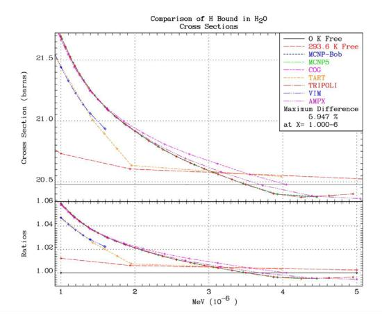
The figure below compares only the seven sets of data used by codes. From this figure we can see a spread in the cross sections of over 6%. The differences are particularly large at low energy, but we also see over 1% differences near the peak of the thermal spectrum, and starting near 0.1 eV up to the joint point near 4 to 5 eV.
