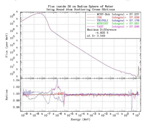
The figure below shows the detailed energy from 1 milli-eV up to 10 eV (10<sup>-9</sup> to 10<sup>-5</sup> MeV). Here we can see the differences in the calculated flux due to how each code handles the bound thermal scattering law data. Note in particular the differences we see in the 1 to 4 MeV energy range of up to +/-4% for MERCURY and TART; more about this below.
