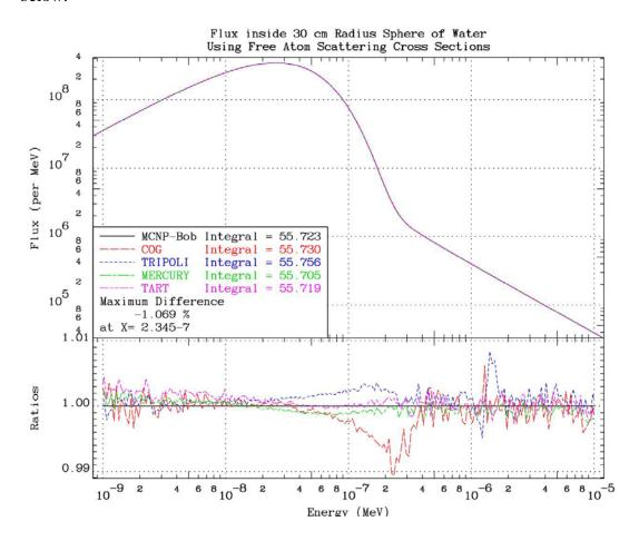
As mentioned above, log scaling can often mask the real magnitude of differences, so below we show the important energy range around the peak of the thermal spectrum. Note that near the peak of the spectrum all of the codes agree very well at the 0.2% level; this indicates that for integral values, such as the reaction rates, even though the energy dependent fluxes differ, all of these codes will produce similar integral results.
