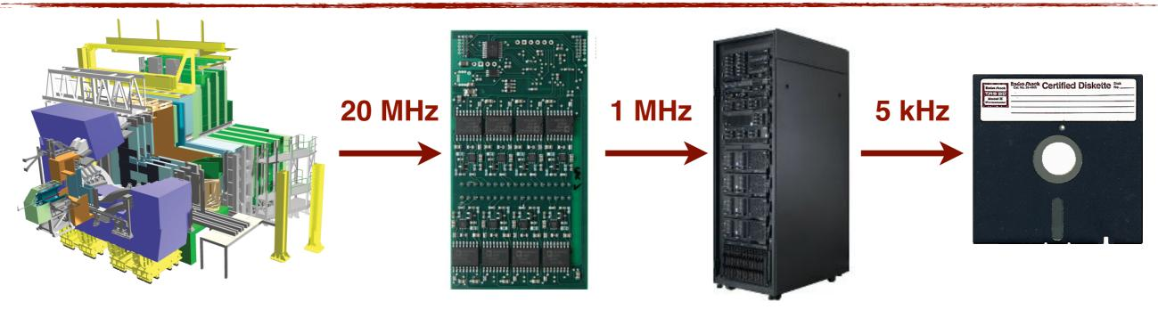
We can "only" read out the detector at 1 MHz; thus, a hardware trigger is required. The basic trigger strategy is
